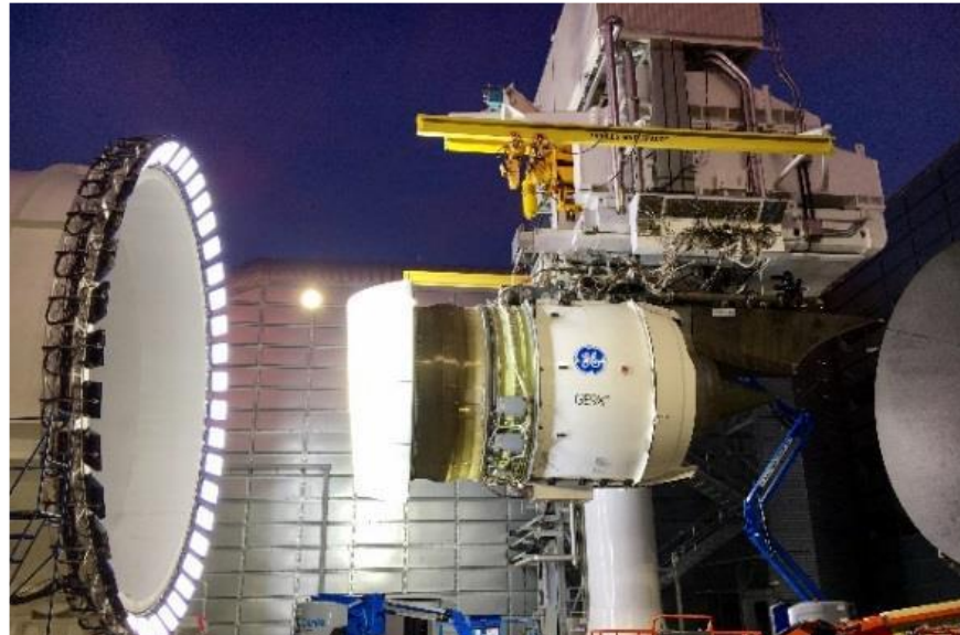
The GE 9X shown here is used on the Boeing 777X and is the largest & highest thrust aircraft engine in the world.
